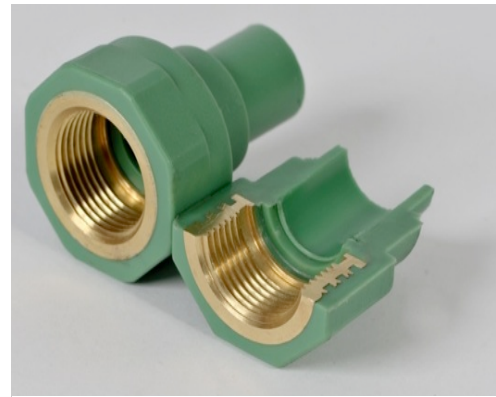
Example of a Non-Fusion fitting that permits transition from PP-R to non-thermoplastic pipe or fitting with threaded connection – courtesy of Pestan
